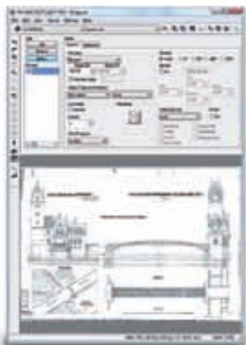
Using RW-3600 PLOTCLIENT/WIN you can change the print settings of supported file formats without the need to launch the application software with which the file was made.
